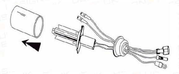
STEP 4: Insert the xenon bulb into the headlight.
